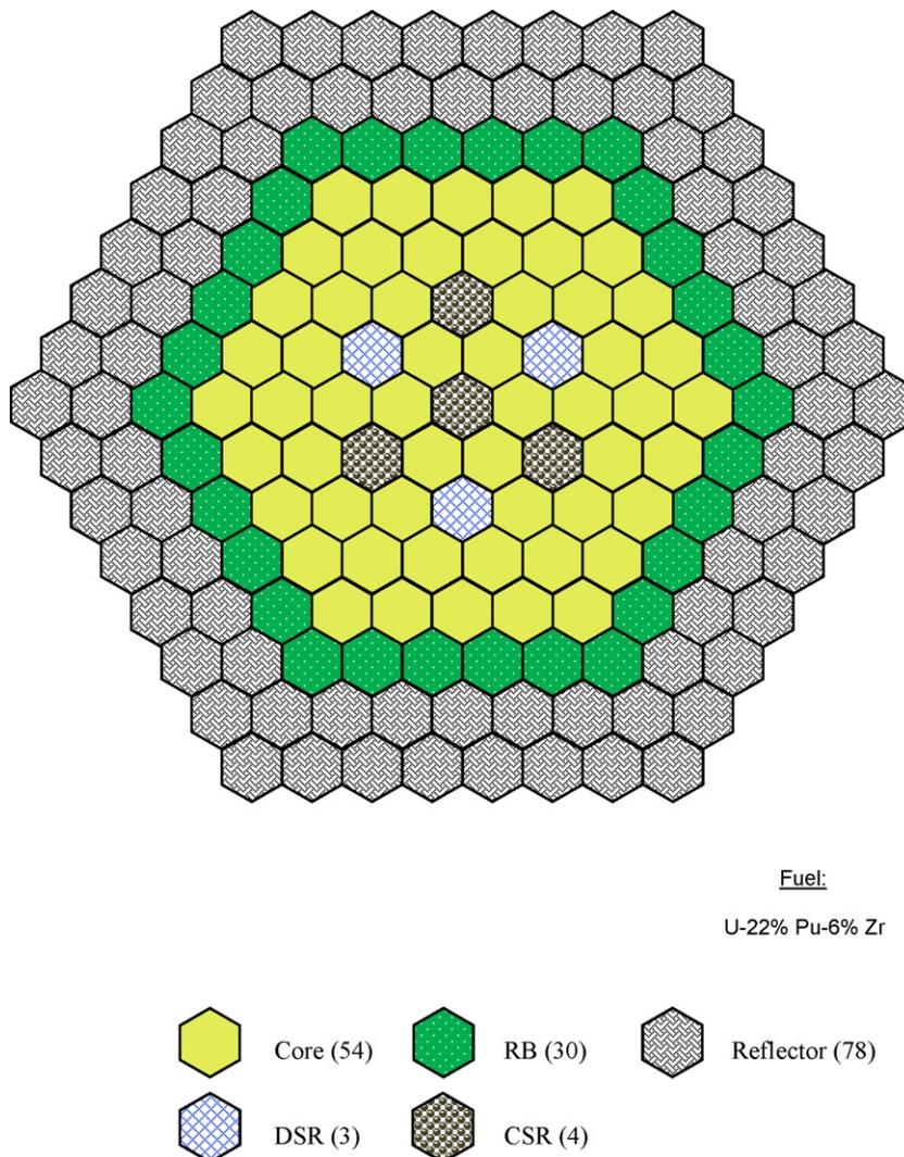
**Fig. 7.** Core configuration of a 320 MWt metal fuelled fast reactor (FBR-4).
