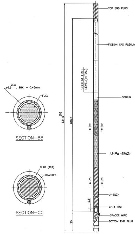
**Fig. 2.** Sodium bonded metallic fuel pin design.
