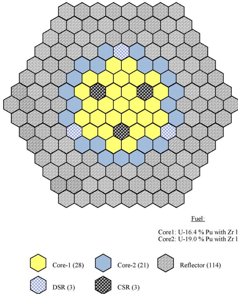
**Fig. 4.** Core configuration of a 300 MWt metal fuelled fast reactor (FBR-1).
