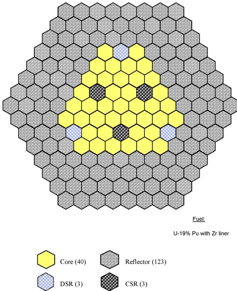
**Fig. 5.** Core configuration of a 220 MWt metal fuelled fast reactor (FBR-2).
