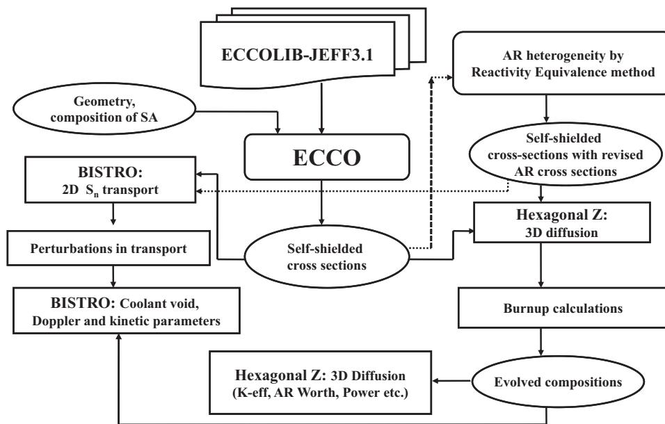
**Fig. 3.** Flowchart of FBR core calculations with ERANOS 2.1 system.
