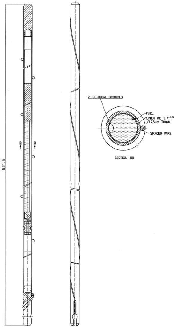
**Fig. 1.** Mechanically bonded metallic fuel pin design.
