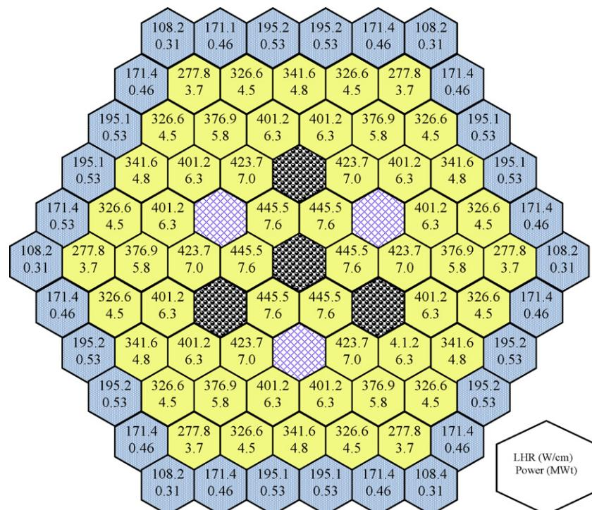
**Fig. 8.** SA power and peak LHR for BOL core of FBR-4 (all rods up): 320 MWt.
