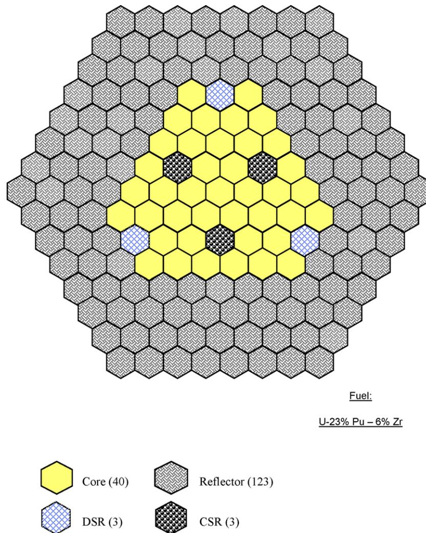
**Fig. 6.** Core configuration of a 220 MWt metal fuelled fast reactor (FBR-3).
